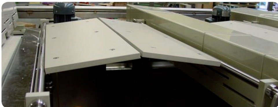
Foamlite® P grey Cover flaps over a galvanic tank
