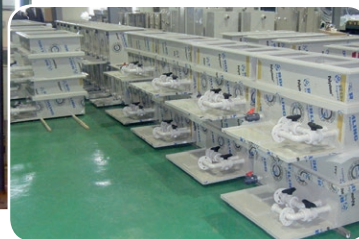
Polystone® P homopolymer grey Tank for a copper-coating plant
