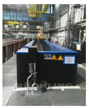
**Exterior cladding made from Polystone® G blue B 100-RC:** The material is suitable for permanent contact with aggressive nitric and hydrofluoric acids and contributes to the plant's high operational safety and performance
