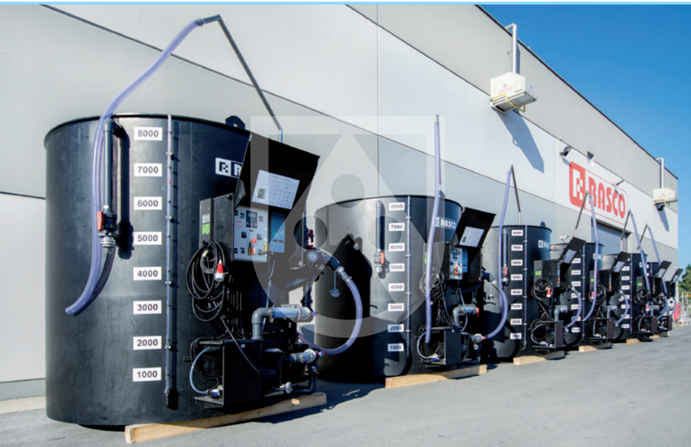
Mixing tanks for liquid salting vehicles: a brine solution is produced with modern technology, based on sodium chloride (NaCl), calcium chloride (CaCl 2 ) or urea
