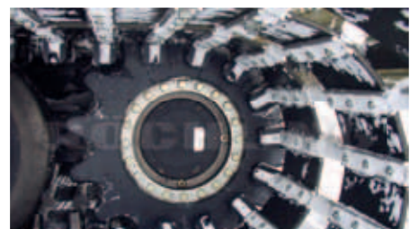
Drive sprocket in an alpine vehicle
