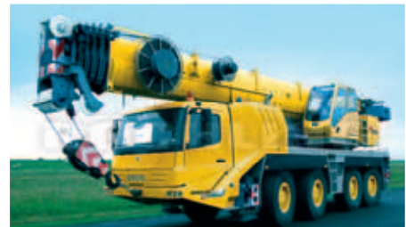
Crane with slide element in boom
