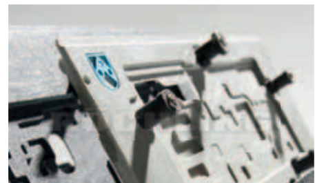
Solder pallet for transport of PC boards
