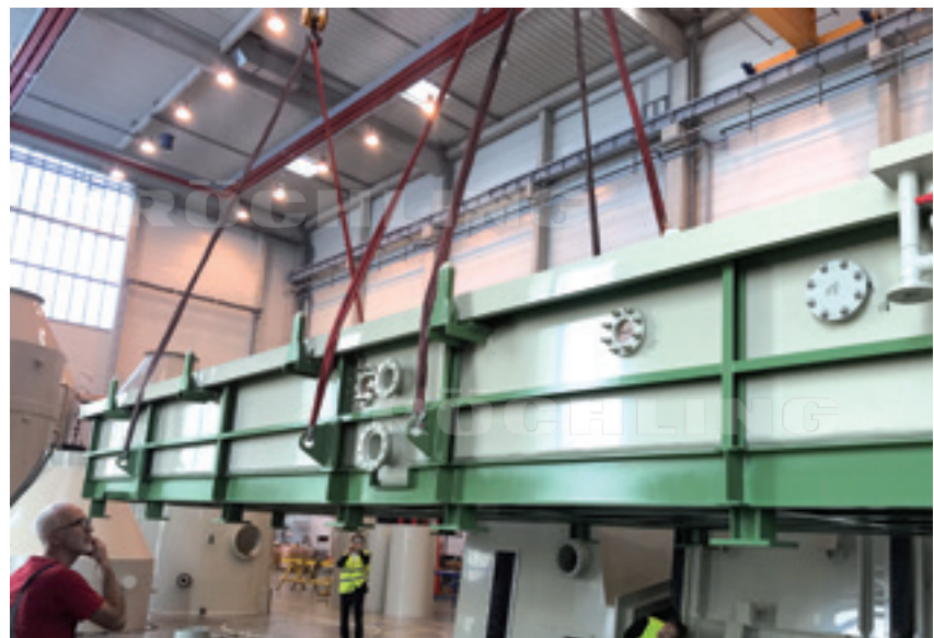
Polystone® P homopolymer grey Extra heat stabilised for a steel-pickling plant
